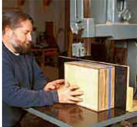
**Saw off the top of the box on a bandsaw. Tape the entire saw line, and use a 1/2-in., 3-tpi blade to avoid breakout.**
