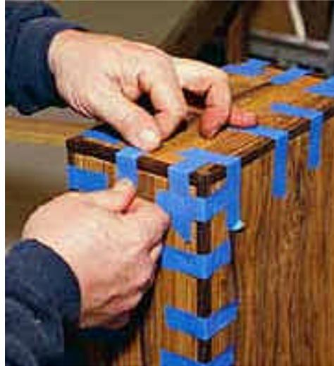
Yellow glue and tape attach the edge-banding. Wenge edge-banding is butted at the corners, not mitered, because end grain is not conspicuous.
