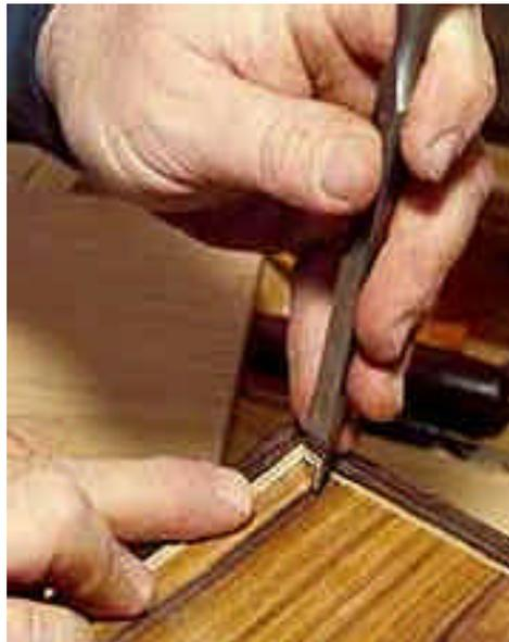
Press the inlay into the groove with the back of a chisel. It should not need clamping or taping. Fine-tune the miter if necessary.
