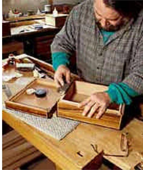
Careful with that bevel angle. It determines the rate the humidor loses humidity and receives fresh air. A humidor that is opened frequently should have a tighter fitting lid.
