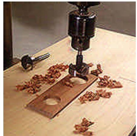
16 -- Bore the holes in the instrument block using a Forstner bit. Enlarge the hole for the humidifier with a drum sander.
