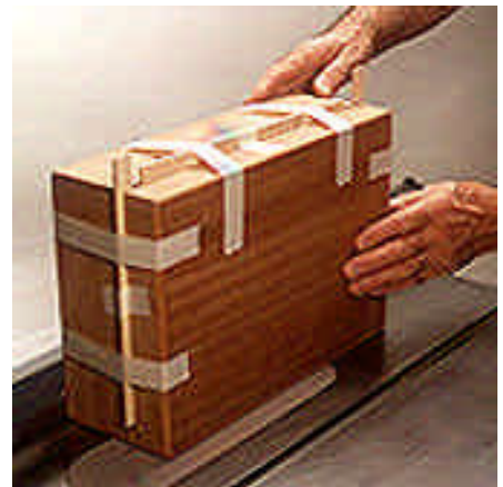
11 -- Cut the lid off the box on the table saw. Tape in a spacer strip to support the lid after making each cut.
