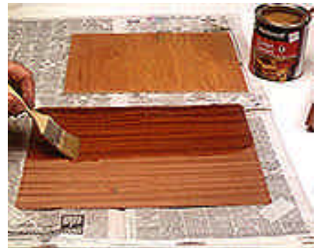
8 -- Evenly apply contact cement to the veneer and the plywood panels, using a small bristle brush.
