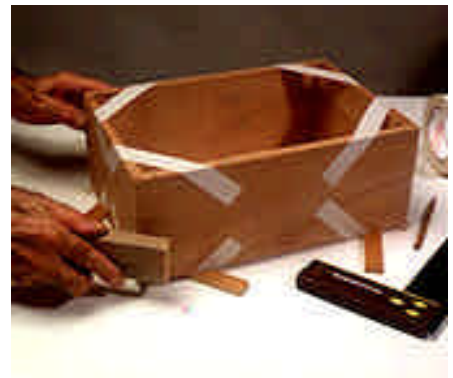
2 -- Test fit the sides and ends. Tape the pieces together and remove the sharp corners by hand sanding.
