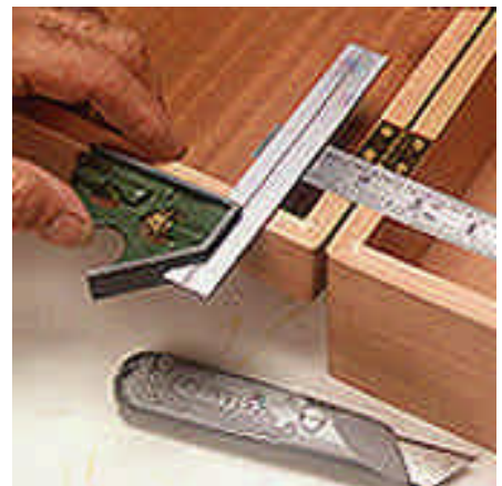
12 -- Use a ruler, square and knife to lay out and mark location of lid-support hole. Measure from the hinge pin's center.
