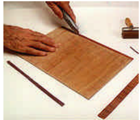
9 -- Use a sharp knife to trim off the excess veneer. Cut from both ends toward the panel's center to prevent tearout.
