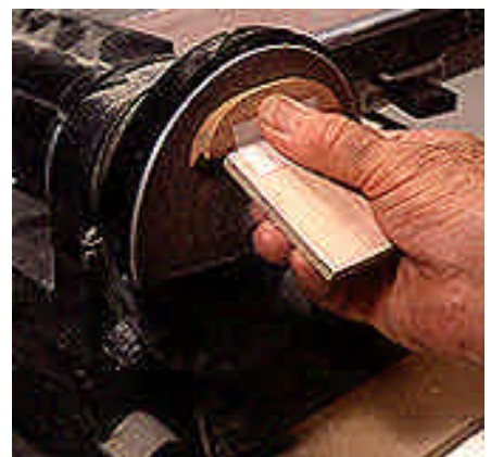
14 -- Cut the curve and notch in the handle pieces, then sand the taper on them, using a disc sander.
