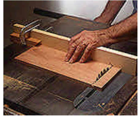
1 -- Cut the miters on the sides and ends, using an auxiliary fence and a 45 degree miter stopblock clamped in place.
