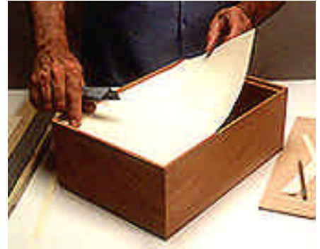
7 -- Make a cardboard template of the top panel. Test it in the rabbet-it should fit in the space snugly.
