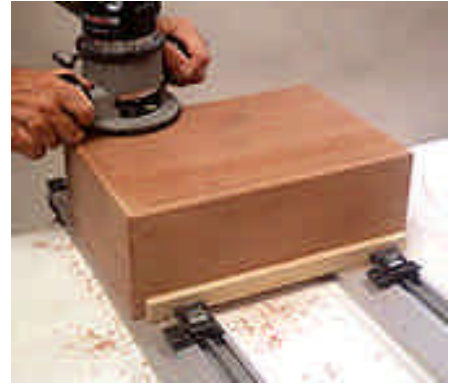
10 -- Using a 3/16-in.-rad. corner-rounding bit in the router, make the crossgrain end cuts before cutting with the grain.
